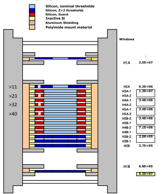
In Stage-4 Dynamic Thresholds all segments of H1A to H3B are raised to respond only to  $Z \ge 6$ . The B-End response to H, He, and electrons is essentially disabled, but the A-End stopping response is retained through most of the stack.
