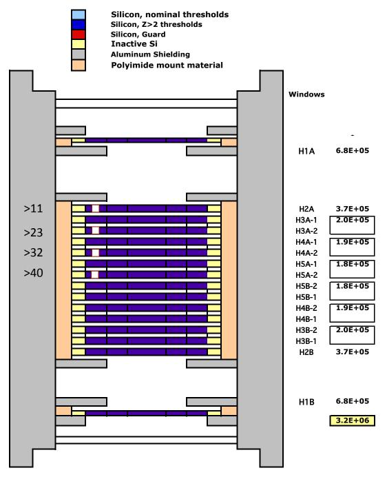
In Stage-7 Dynamic Thresholds we rely entirely on the Pixels to get proton spectra (see approximate thresholds). We start out with all 4 pixels active but may have to raise the pixel trigger thresholds above that of protons (e.g., to ~15-20 MeV in a 1-mm thick detector) if the singles rates remain too large. We would start by raising the threshold only on the H2A pixel, and continue as needed.
