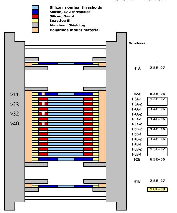
In Stage-3 Dynamic Thresholds all outer segments of H1A and H1B are raised to respond only to Z≥6. The H, He, and electron energy range is the same with a reduced geometry factor.
