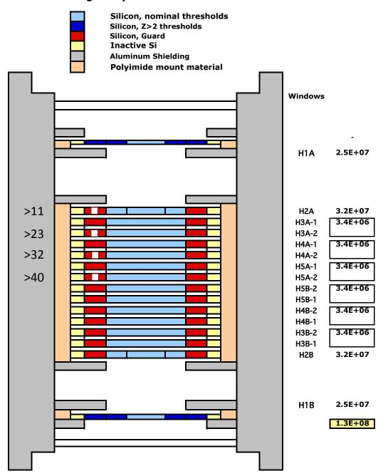
In Stage-2 Dynamic Thresholds the outer segments of H1A and H1B are also raised to respond only to  $Z \ge 6$ . Thus the geometry factors for H, He, and  $e^-$  are reduced by a factor of ~5. The geometry for  $Z \ge 6$  ions remains at the original level.
