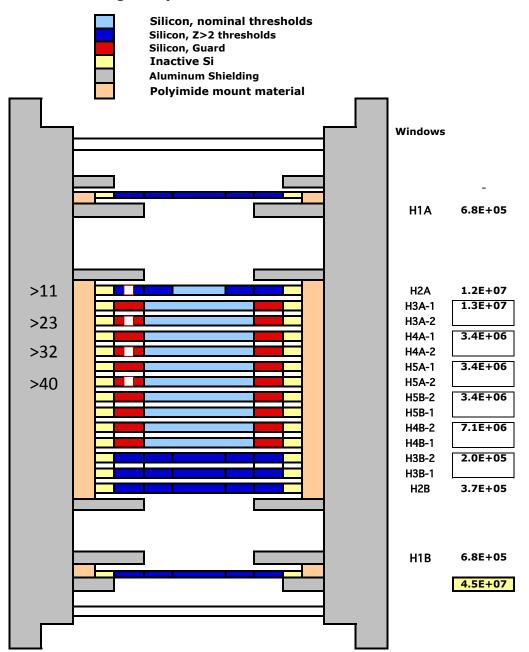
This Stage-5 concept is a minor change from Stage-4. The only difference is that the threshold for the center of H2B has been raised. The B-End response to H, He, and electrons is essentially disabled, but the A-End stopping response is retained through most of the stack. The center of H2A would be required for all H, He, and electron events.
