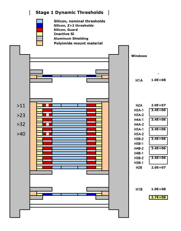
In Stage-1 Dynamic Thresholds the guard regions of the H1A and H1B devices are raised to respond only to  $Z \ge 6$  (see legend for color coding). Thus the H1 singles rates can be dropped by a factor of almost 3, but there will be more "edge effects" in the outer H1 segments.
