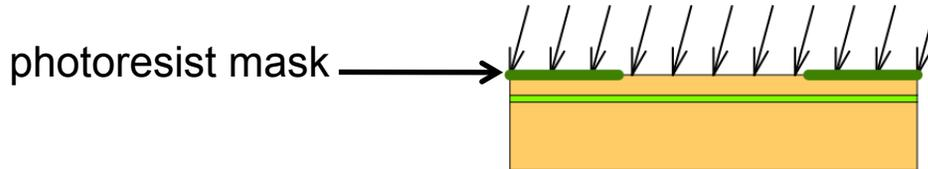
ion implant to produce diode pn junctions on device layer
