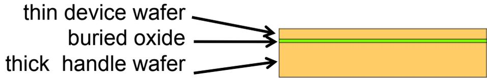
silicon-on-insulator (SOI) wafer is a commercial product with excellent device layer uniformity and control
