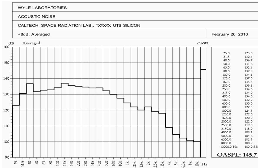
highest test level: 145 dB = Atlas V level + 7 dB
