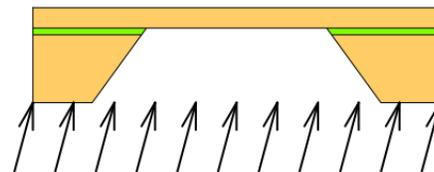
ion implant from back to produce detector's ohmic contact
