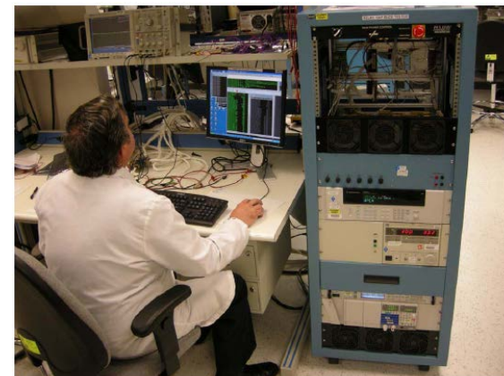
PDU Resistor/Capacitor Slice Testset
