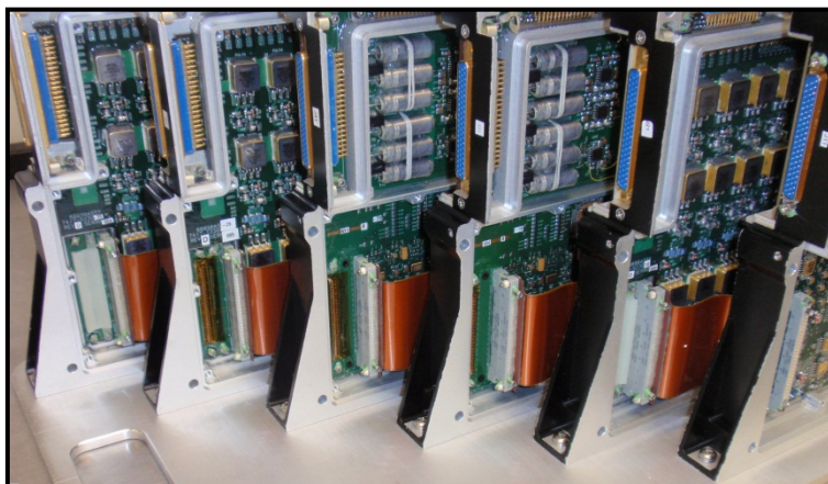
Detail of slice-to-slice connection. Installation fixture used to hold slices.
