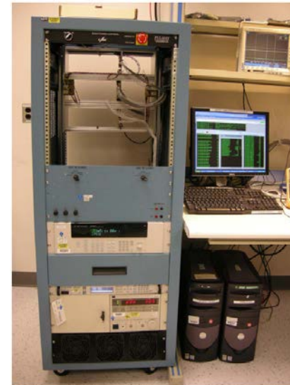
PDU Command/Telemetry Slice Testset
