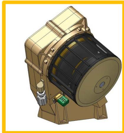
SPAN-B on anti-ram side looks "behind" spacecraft motion
